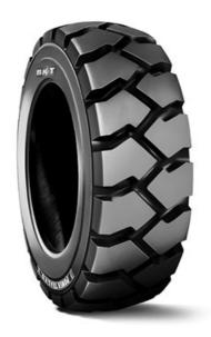
POWER TRAX HD is a premium bias-ply tire that is specially designed for forklift equipment in industrial applications. The deep tread, the extra thick sidewall and the tough casing provide exceptional durability minimizing the risk of punctures and accidental damages. The tire features excellent cut, chip and tear resistance suitable for rough and hard concrete surface. The specially designed rim guard ensures protection
