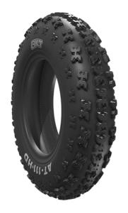
Description AT 111 HD is suitable for all-terrain sport racing with ATVs. The increased tread depth and the thick sidewall
