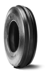
**Description** TF 9090 is a tire designed for small tractors in soil tillage
