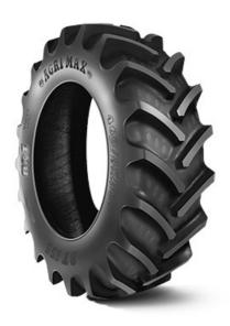
**Description**AGRIMAX RT 855 provides excellent traction and comfort properties. Mainly designed for soil tillage and both field and road transport, some sizes are also suitable for
