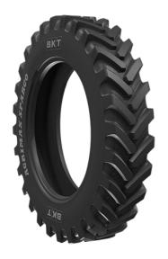
AGRIMAX SPARGO is the special BKT tire for row crop applications. It has been designed for enhanced productivity in the fields and for preserving the soil in the long term. Thanks to VF technology, the tire provides higher load capacity at standard pressure. Thanks to a strong casing and an increased number of lugs, AGRIMAX SPARGO ensures outstanding durability along with strong stability both in the fields and during road
