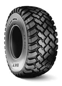
RIDEMAX FL 690 is a radial flotation and transport tire for tank trucks and trailers. The tire is suitable for 75% on-the-road applications. As a response to the increasing demand for high loads in modern agriculture, BKT has designed this steel-belted tire withstanding very heavy loads and increasing the farmer's productivity. The low rolling resistance contributes to better fuel economy.
